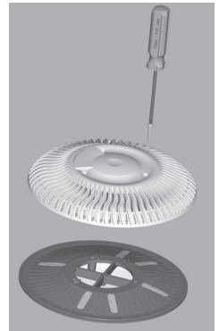
Fig. 11: Attach SDX RETRO Drain Cover
