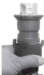
Place the nozzle inside the nozzle tool to hold it from spinning as you twist on the cap.
