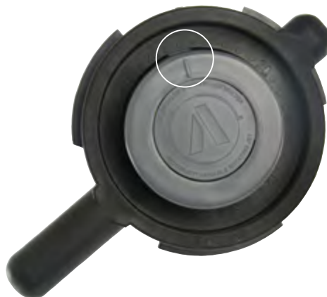
Fig. 12: Aiming mark lined up with number on tool
